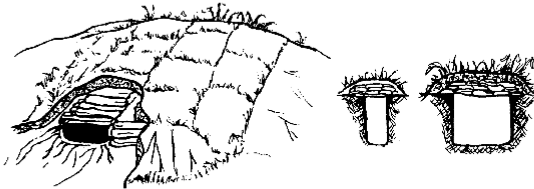
Figure 4-6. Sandbags protected with sod and earth cover.
